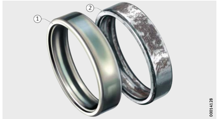
Figure 7 Bearing rings after the salt spray test
