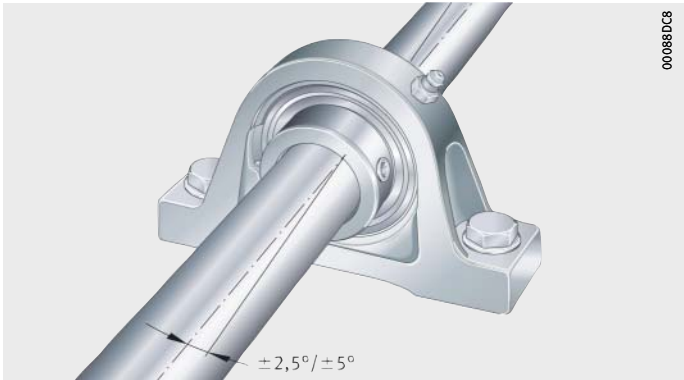
Figure 1 Compensation of static shaft misalignment
